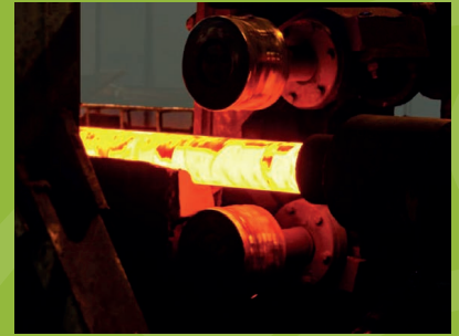
Hot rolling mill
